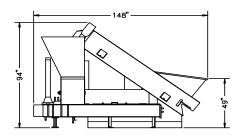
DAC 1200 with Optional Conveyor/Separator - side view
